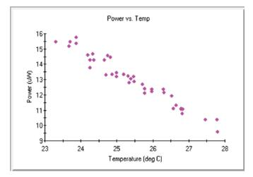
Figure 5. Change in optical power of the 980 nm laser diode as a function of temperature.
