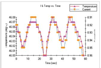
Figure 6. The steady state temperature of the nonlinear crystal package, controlled at 46 deg C.
