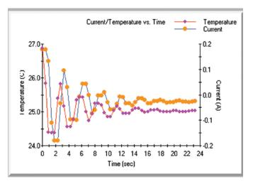
Figure 4. A plot of the temperature and current vs time, showing the transient fluctuations of the temperature, measured on a butterfly packaged 980 nm laser diode.
