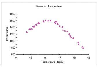
Figure 7. A P vs. T plot of the 490 nm intensity of a SHG crystal waveguide.
